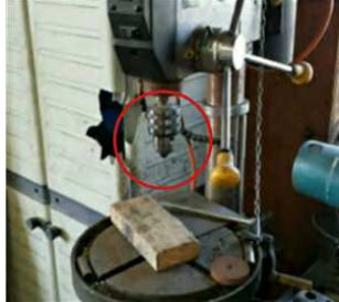
Chuck guard needed on drill press
