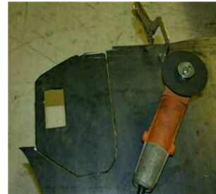
Guard missing on grinder
