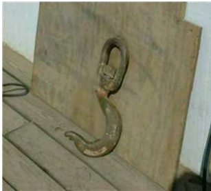
Damaged hook in fab area
