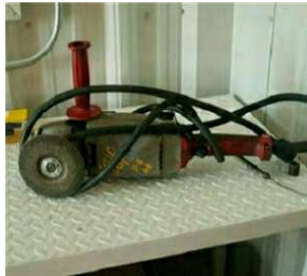
Guard missing on angle grinder
