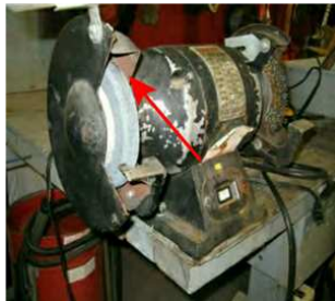
Tongue guard missing
