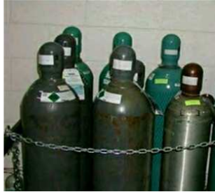
Proper Cylinder storage
