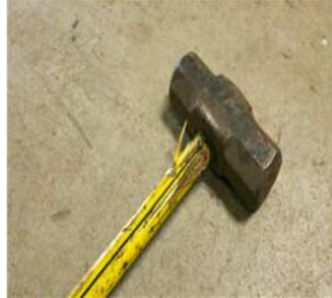
Damaged shaft on hammer
