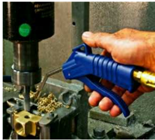
Non approved air nozzle in fab shop
