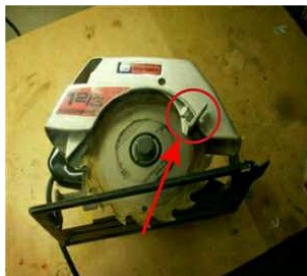
Self-adjusting guard is bypassed
